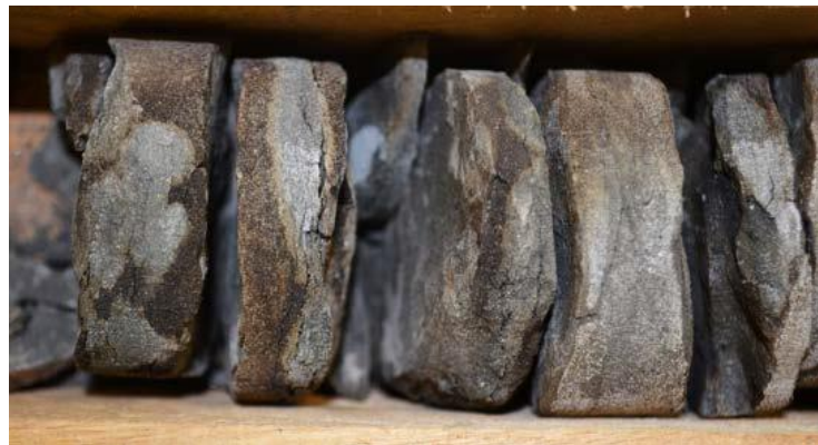
Fig. 23 – Oil stains in Cerrezuelo sandstones (Devonian) from core of Achar E-1 stratigraphic well. Taken from Petrel web page (published in Energy Oil and Gas Conference, Sydney 2015)
